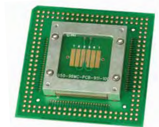
Bottom of 950-096 mini card shown here with contacts for heated socket base
