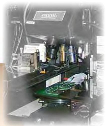
950-096 Dedicated Fixture Mounted on a RTI MultiTrace Test System and Connected to a Black Box For Microscope Use
