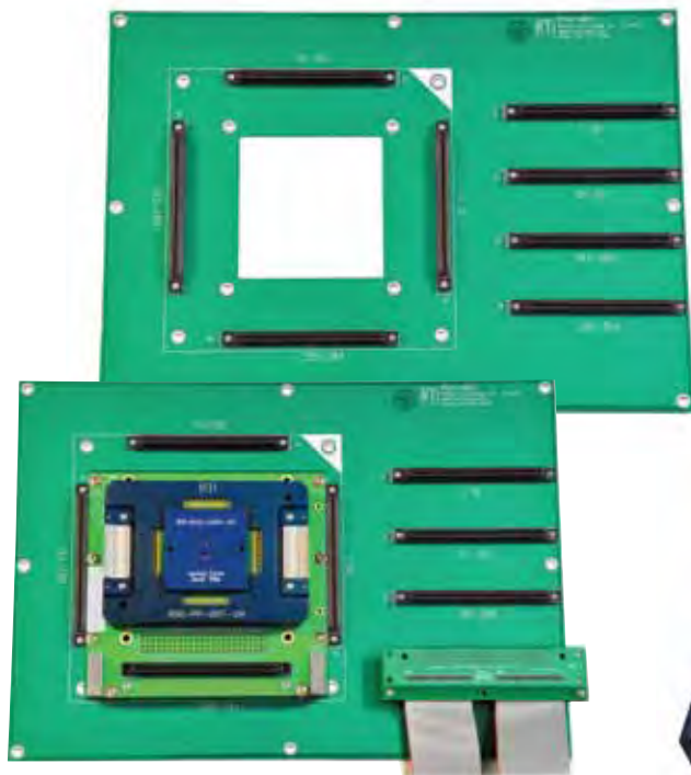
950-096 Fixture Mounted on a 950-384 Connector Motherboard
