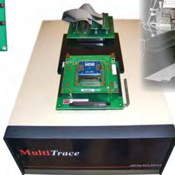
950-096 Fixture Mounted on a 950-384 Connector Motherboard
