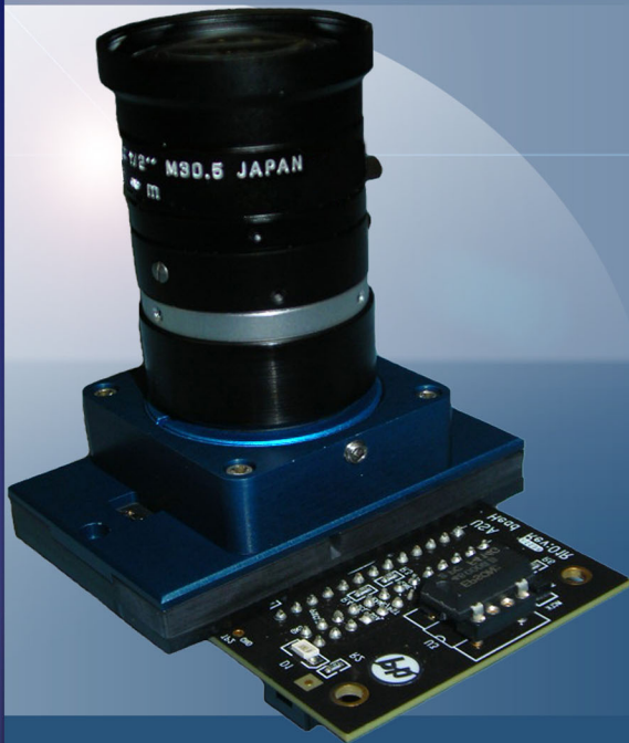
Custom Socket for Evaluation of Optical Chip with Adjustable Lens Lid
