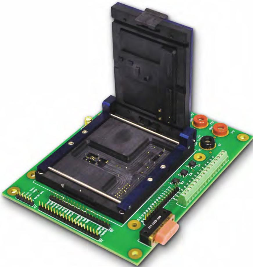
Custom breakout benchtop fixture for Rigid Flex MCM device includes variety of header pins, terminals and standard connectors
