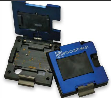
Module test socket with custom pin position and opening for access to MCM on-board connector
