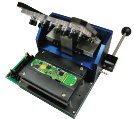
Singulated MCM sensor module in 750 series test press with breakout to connectors of choice
