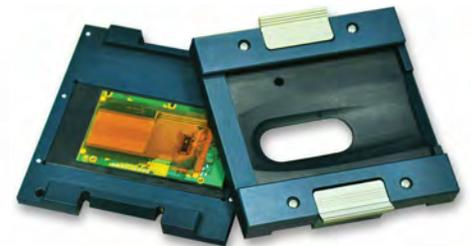
Sensor module with physical access for functional test and cutouts for SMT components
