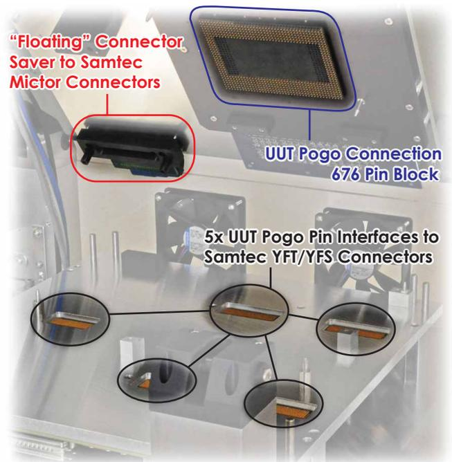
*A Few Contact Sites That Mate With Connectors on the Final Board Under Test*
