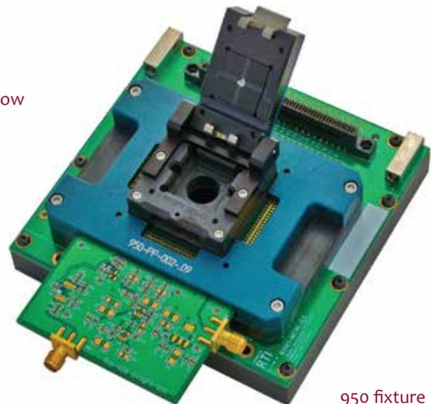
950 fixture with modified daughter card to allow RF measurements on a hybrid RF module.
