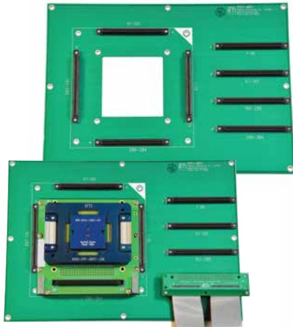
950 Fixture Mounted on a 950-384 Connector Motherboard
