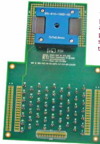
Extended daughter card with header pins and plated thru holes to allow access to all DUT pins. Can be used stand-alone or with the 950 base.
