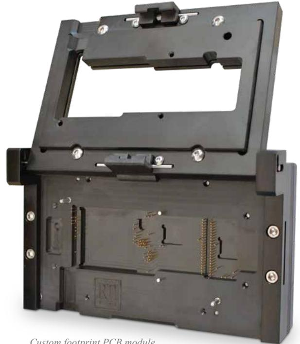
*Custom footprint PCB module test socket body with a hinged dual latch lid uses multiple guide pins for precise UUT alignment*
