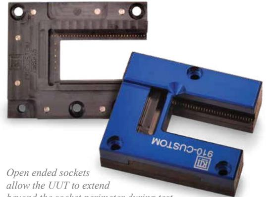
Open ended sockets allow the UUT to extend beyond the socket perimeter during test
