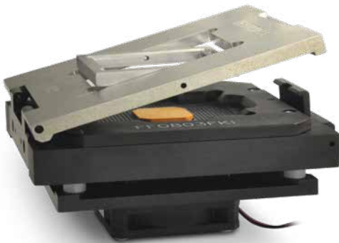
A pivoting pressure plate on a single axis gimbal provides evenly distributed vertical compression force against the DUT as the clamshell lid is closed, preventing damage to all contacts
