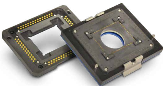
Lids including an interposer PCB and pogo pins can contact test points located on the same side of a CMOS image sensor that needs topside access and exposure during test. Signals are routed through the lid and back down through the test socket body to the DUT board.
