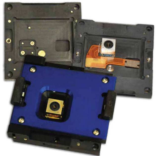
Relief cutouts in the socket base provide room for components installed on the UUT and very fine pitch pogo pins can contact high speed connectors installed on Rigid and Rigid-Flex PCB modules
