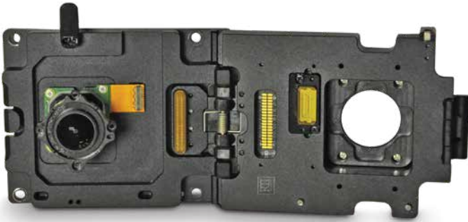
Fully custom test sockets include a combination of interposers, connector savers, relief cutouts, and multi-stage alignment/closing processes when needed
